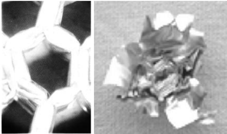
Fig3. (a) Crushed aluminum honeycomb core near the penetrated region (b)Produced plug from aluminum honeycomb core at 94 m/s impact velocity
