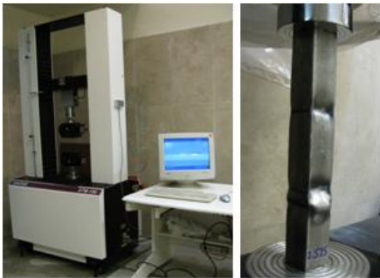
Fig3. Tensile and pressure test equipment and placement of sample under pressure
