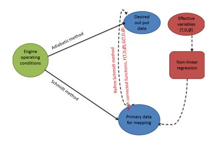
Fig1. Schematic of the proposed approach to modeling SE
