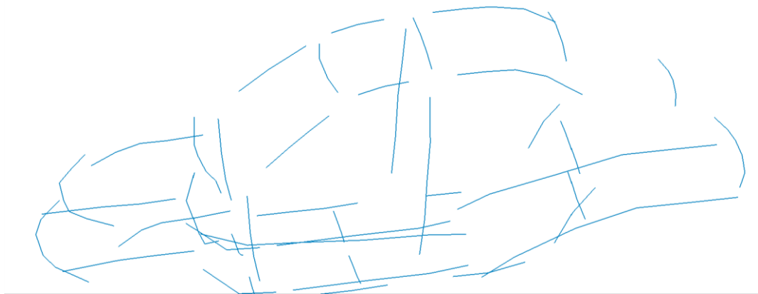
Fig3.: Equivalent beam modeling of the BIW
