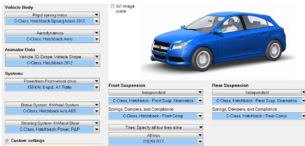
Figure13: CarSim vehicle's configuration part
