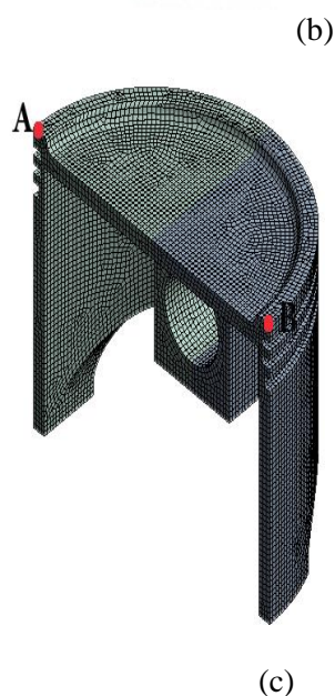
Figure 1. The piston used in the FE analyses: a) gasoline engine b) the piston, c) meshing of the FE model.
