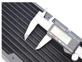
Figure 3: Radiator fin density
