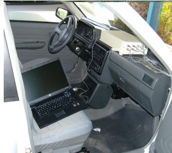
Figure 7: The data acquisition system and temperature sensors
