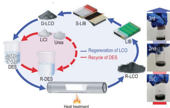
Figure 15: Eutectic solvent use cycle [74]
