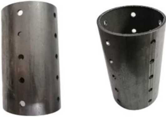
Figure 2: The perforated test specimen
