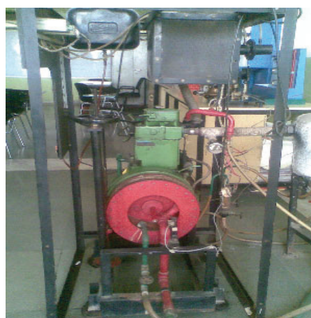
Plate 2. Rope Brake Dynamometer
